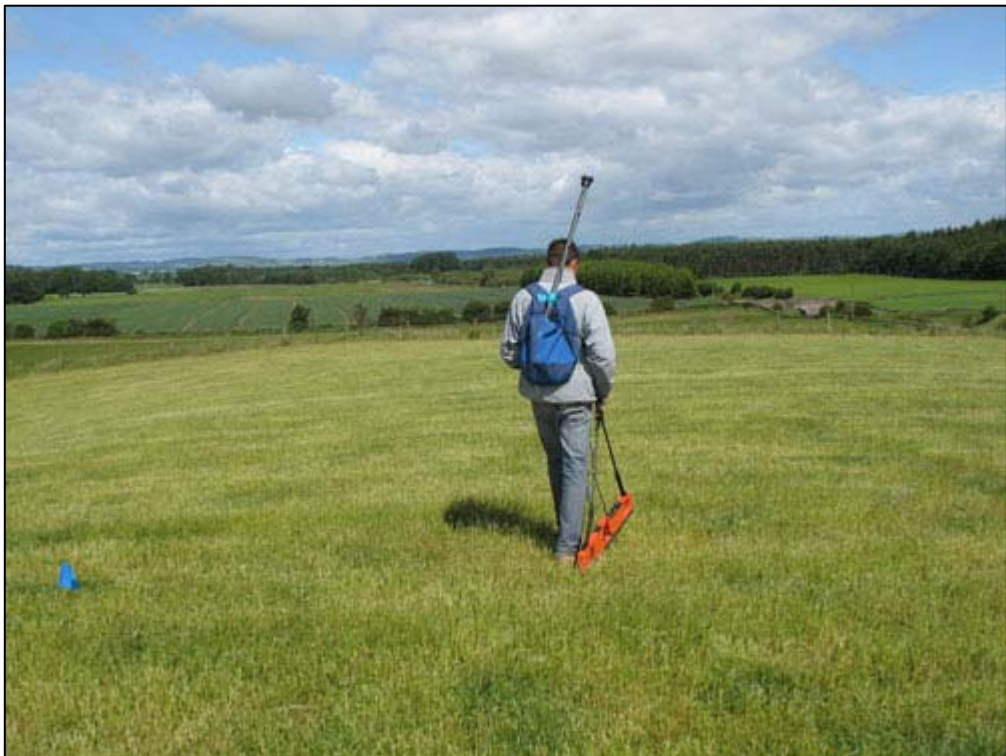
Figure 5b: Geophysics being undertaken with a GEM Proton Magnetometer
